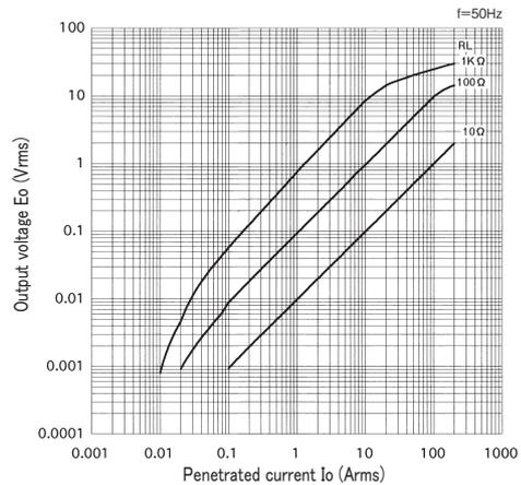
**[Coupling efficiency (K) characteristics]**
