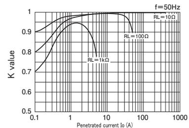
( Possible to calculate output voltage with reading (K) from load resistor and penetrated current )
