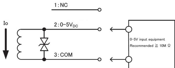
※ Recommend ≤ 1m for cable length (1m extension cable as accessory)
