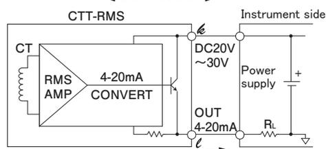
2 wires transmission method in common of (+) power supply of instrument
